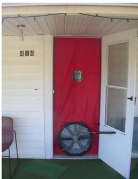
Diagnostic tools, like the blower door shown here, are used in weatherization to identify areas of air infiltration.
